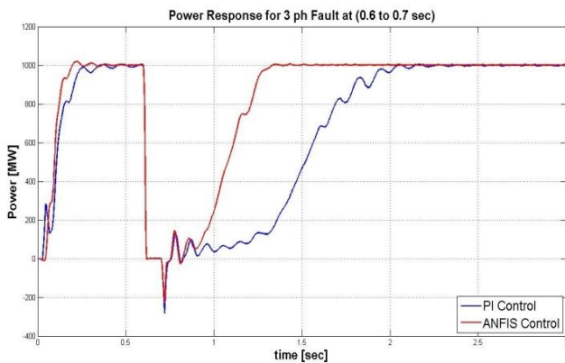
Fig. 21: Active power when a three-phase fault occurs.
